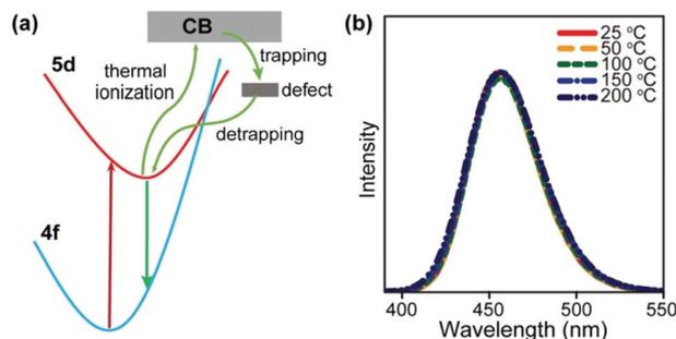
**Fig. 8** (a) A simplified model for the zero-thermal-quenching due to structural defects. (b) Temperature-dependent emission spectra of  $\text{Na}_3\text{Sc}_2(\text{PO}_4)_3:\text{Eu}$  (divalent, 0.7%) phosphors under 370 nm excitation in the temperature range of 25–200 °C. Reproduced with permission from ref. 104. Copyright 2017, Nature Publishing Group.
