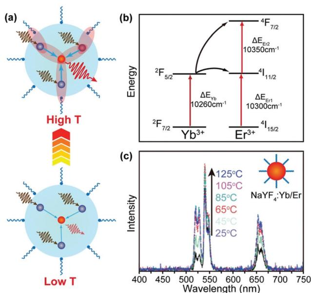
**Fig. 6** (a) Thermal activation of phonon-assisted energy transfer. (b) Mismatch of energy levels between Yb<sup>3+</sup> and Er<sup>3+</sup> ions, illustrating the need for phonon participation in the energy transfer process. (c) Temperature-dependent upconversion emission spectra of NaYF<sub>4</sub>:Yb/Er (20/2%) UCNPs (24 nm) in the temperature range of 25–125 °C. Reproduced with permission from ref. 79. Copyright 2014, American Chemical Society.
