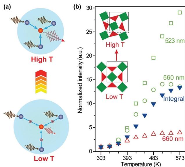
**Fig. 7** (a) Thermal promotion of energy delivery to activator ions by lattice contraction in negative thermal expansion crystals. (b) Normalized emission intensities of Yb<sub>2</sub>W<sub>3</sub>O<sub>12</sub>:Er (6%) nanocrystals as a function of temperature. Inset: schematic of the lattice contraction and distortion as the temperature increases. Adapted with permission from ref. 101. Copyright 2019, Wiley-VCH.
