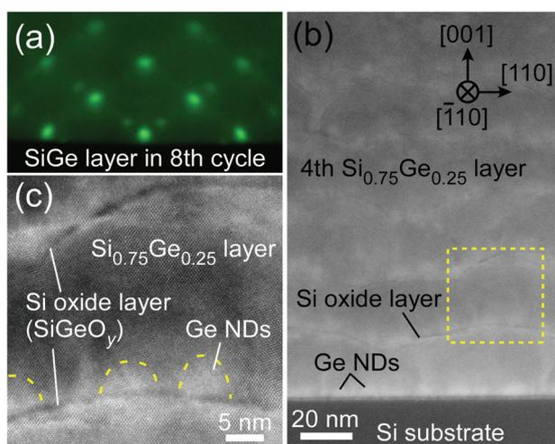
**Fig. 2** (a) RHEED pattern of the  $\text{Si}_{0.75}\text{Ge}_{0.25}$  layer in the 8th cycle structure of the Ge ND ( $\sim 8$  nm)/ $\text{Si}_{0.75}\text{Ge}_{0.25}$  ( $\sim 22$  nm) film. (b and c) Cross-sectional ADF-TEM images of the Ge ND ( $\sim 8$  nm)/ $\text{Si}_{0.75}\text{Ge}_{0.25}$  ( $\sim 22$  nm) film: (b) low and high (c) magnifications. The image in (c) corresponds to the region marked by the dotted square in (b).
