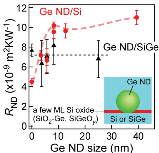
Fig. 4 The Ge ND size dependence of  $R_{\text{ND}}$  of the Ge ND/Si films (the red circles) and the Ge ND/ $\text{Si}_{0.75}\text{Ge}_{0.25}$  films (the black triangles). The dashed and dotted curves are the eye-guides.
