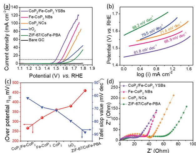
Fig. 7 (a) Linear sweep voltammetry curves of different electrocatalysts. (b) Corresponding Tafel slopes. (c) The required overpotential to achieve a current density of  $10 \text{ mA cm}^{-2}$  and Tafel slope values for different catalysts. (d) Corresponding EIS Nyquist plots.
