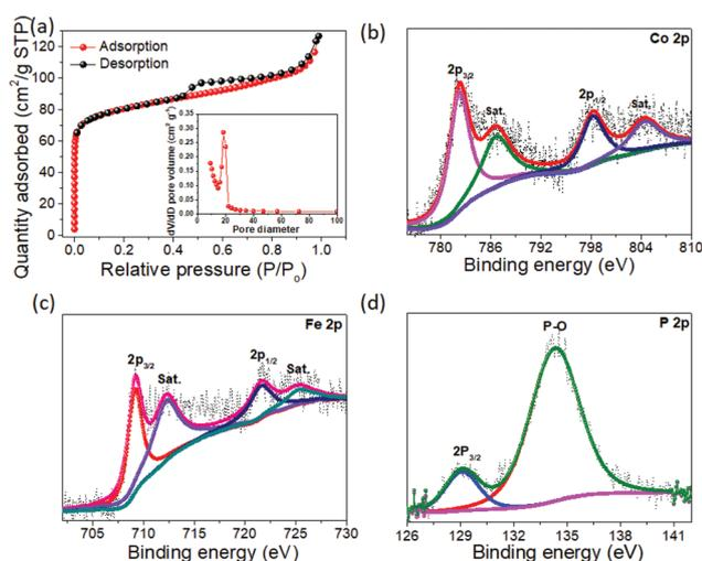
Fig. 5 (a) Nitrogen adsorption–desorption isotherm (the inset shows the pore size distribution curve) for  $\text{CoP}_2/\text{Fe-CoP}_2$  YSBs. (b) High-resolution XPS spectra of  $\text{Co } 2\text{p}$ , (c)  $\text{Fe } 2\text{p}$  and (d)  $\text{P } 2\text{p}$  for  $\text{CoP}_2/\text{Fe-CoP}_2$  YSBs.
