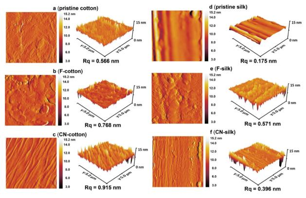
Fig. 3 AFM topology and 3D images (5 × 5 µm) of (a) pristine cotton, (b) F-cotton, (c) CN-cotton, (d) pristine silk, (e) F-silk and (f) CN-silk.
