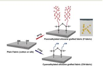
Fig. 1 Schematic illustration of the surface chemical modification of natural textiles with different silanes and a photograph of droplets of water on F-cotton.
