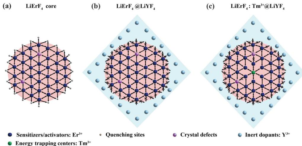
**Fig. 3** (a) The energy migration quenching processes in a  $\text{LiErF}_4$  UCNP. (b) A typical strategy to reduce the energy migration to surface quenching sites through an inert-shell coating. (c) The approach of simultaneously preventing energy migration quenching processes through introducing  $\text{Tm}^{3+}$  ions as energy trapping centers.
