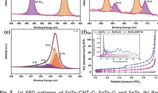
Fig. 3 (a) XRD patterns of SnTe-CNT-G, SnTe-G and SnTe. (b) Raman spectra of SnTe-CNT-G, SnTe-G and SnTe. Core-level XPS spectra of Sn 3d (c), Te 3d (d) and C 1s (e). (f)  $\rm N_2$  adsorption and desorption isotherm curves of all samples, where the inset shows the pore-size distribution.
