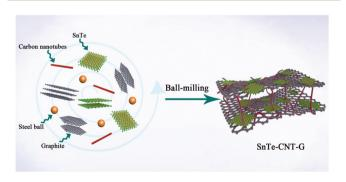
**Fig. 1** Schematic illustration of the SnTe-CNT-G composite synthesis process.
