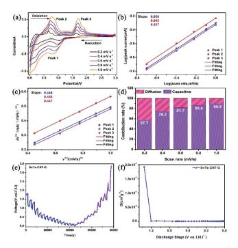
Fig. 5 (a) CV curves obtained at different scan rates. (b) The corresponding  $\log(i)$  versus  $\log(v)$  plots and (c) the corresponding  $i/v^{1/2}$  versus  $v^{1/2}$  plots of the SnTe-CNT-G electrodes. (d) The normalized ratio of the capacitive- and diffusion-controlled contributions at different scan rates. GITT curves of the SnTe-CNT-G electrode (e) and their Li<sup>+</sup> diffusion coefficient for the initial discharge states (f).
