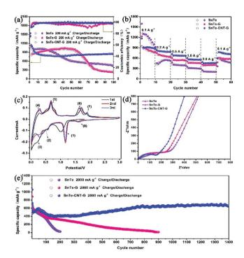
**Fig. 4** (a) Cycling performance and coulombic efficiency of the three samples at 200 mA  $\rm g^{-1}$ . (b) Rate performance of all samples. (c) CV curves of the SnTe-CNT-G anodes at 0.2 mV  $\rm s^{-1}$ . (d) Nyquist plots of all electrodes before cycling. (e) Cycling performance at 2000 mA  $\rm g^{-1}$ .
