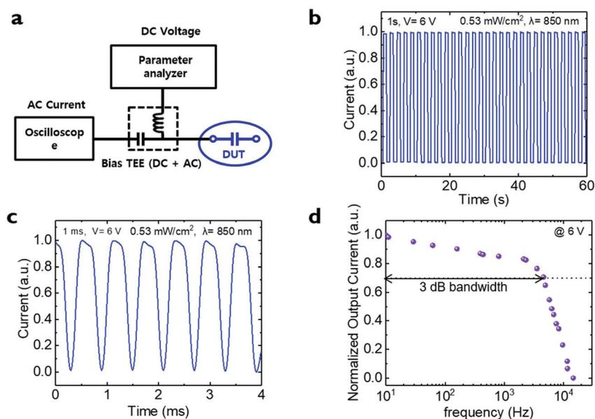
**Fig. 5** (a) Schematic diagram of experimental setup for dynamic AC photocurrent measurements. (b and c) Dynamic photoresponse of the MoS<sub>2</sub>/Si photodetector under repeated on/off laser (850 nm) with a timescale of 1 s and 1 ms (1 kHz). (d) Frequency dependence of normalized output current and 3 dB bandwidth of the device at 6 V bias.
