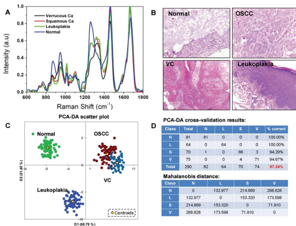
**Fig. 12** (A) Shows the averaged SERS spectra of the various types of oral cancer malignant CTCs compared with normal cells. (B) Optical images of histology stained tissue from various types of cancer and normal samples. (C) 2D scatter plot showing the efficient classification of various cancers from normal. (D) PCA-DA cross-validation results. Reproduced with permission from ref. 144. Copyright 2019, WILEY-VCH Verlag GmbH.
