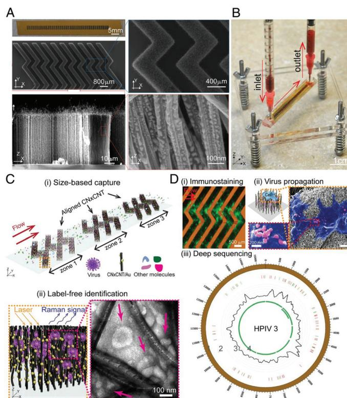
**Fig. 10** Schematic of the working principle of VIRRON platform, including (A) images of aligned CNTs decorated with gold nanoparticles and (B) assembled VIRRON device, (C) illustration of virus capture and label-free Raman identification, and (D) on-chip analysis and enrichment of virus for NGS. Reprinted with no changes from ref. 122, image licensed under <http://creativecommons.org/licenses/by/4.0/>.
