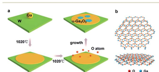
**Fig. 1** (a) Schematic of the  $\alpha$ -Ga<sub>2</sub>O<sub>3</sub> structure growth process. A drop of liquid Ga is placed on a W substrate. Then the Ga forms a flat surface owing to the good wetting behavior between Ga and the substrate as the temperature is increased. The O atoms diffuse to the surface of the liquid Ga to react and form hexagonal-shaped  $\alpha$ -Ga<sub>2</sub>O<sub>3</sub>. (b) Crystal configuration of an  $\alpha$ -Ga<sub>2</sub>O<sub>3</sub> flake.
