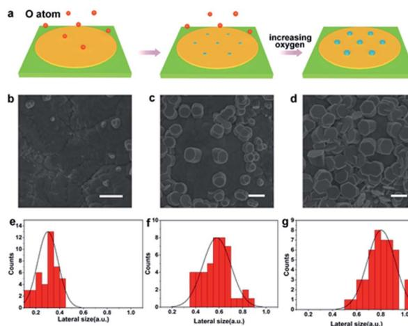
Fig. 3 The shape evolution of the Ga<sub>2</sub>O<sub>3</sub> that grows vertically. (a) Schematic showing the vertical growth mechanism of Ga<sub>2</sub>O<sub>3</sub>. (b–d) SEM images of vertical growth of hexagonal Ga<sub>2</sub>O<sub>3</sub> crystals. (e–g) Lateral size distributions of the Ga<sub>2</sub>O<sub>3</sub> crystal grown on Ga. The scale bars in (b), (c) and (d) are 1 μm.
