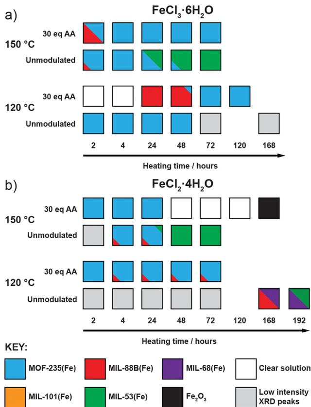
Fig. 3 Crystallisation diagrams for syntheses with (a)  $\text{FeCl}_3 \cdot 6\text{H}_2\text{O}$  and (b)  $\text{FeCl}_2 \cdot 4\text{H}_2\text{O}$  across different times and temperatures, with and without 30 eq. acetic acid modulator. Diffraction data corresponding to the figure can be found in Fig. S12–S15 (part a) and S16–S22 (part b) (ESI†).
