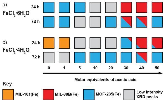
Fig. 2 Crystallisation diagrams for syntheses with (a)  $\text{FeCl}_3 \cdot 6\text{H}_2\text{O}$  and (b)  $\text{FeCl}_2 \cdot 4\text{H}_2\text{O}$ , for both 24 and 72 hours at  $120^\circ\text{C}$  at each modulator concentration. Diffraction data corresponding to the figure can be found in Fig. S2, S3 (part a) and Fig. S4, S5 (part b) (ESI†).
