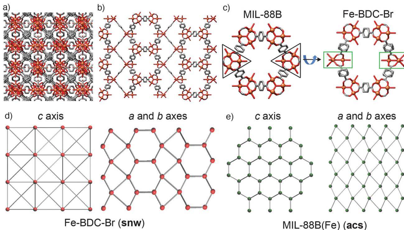
Fig. 5 (a) Crystal packing in the solid-state structure of Fe-BDC-Br as viewed down (a) the  $c$  axis, and (b) the equivalent  $a$  and  $b$  axes. (c) The relationship between the hexagonal units with respect to SBU orientation in the crystal structure of Fe-BDC-Br compared to MIL-88B. Disordered Br atoms in Fe-BDC-Br and H atoms in both removed for clarity. Topological representations of (d) Fe-BDC-Br (**snw**) compared to (e) MIL-88B(Fe) (**acs**).
