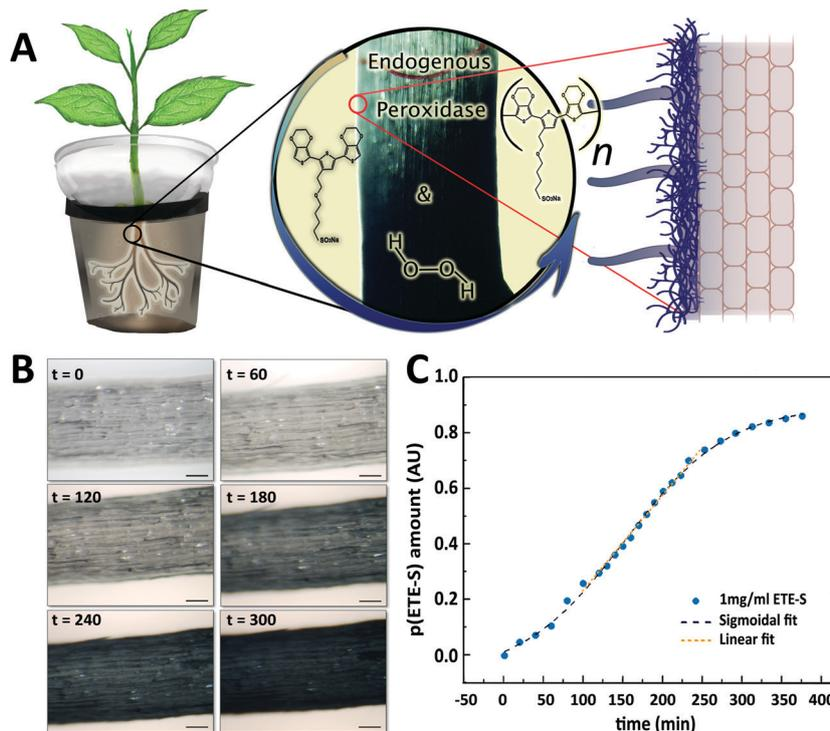
**Fig. 1** Electronic functionalization of plant roots (A) ETE-S polymerizes on the roots of intact bean plant catalyzed by endogenous plant cell wall peroxidases and H<sub>2</sub>O<sub>2</sub>. (B) Micrographs of the root during ETE-S polymerization at different time points from the onset of the reaction (timescale: minutes, scalebar: 100  $\mu$ m). (C) Temporal evolution of p(ETE-S) amount on the root.
