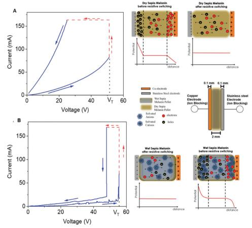
Fig. 8 Resistive switching behaviour at a voltage scan rate of 100 mV s<sup>-1</sup> of (A) dry and (B) wet Sepia melanin pellets in a sandwich configuration between copper and stainless-steel electrodes. Insets in (A) and (B), respectively, show the formation of electronic and ionic (protonic) double layers under bias, leading to resistive switching in both cases. (Reproduced and adapted from ref. 67, copyright (2020) American Chemical Society (ACS)).
