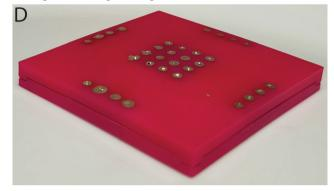
Fig. 1 (A) CAD model of MEA including cutouts on the bottom half and extrusions on the top half in the corresponding positions to clip the halves together, ensure alignment of the electrodes and ensure the MEA could be handled easily in the laboratory. (B) Top view of CAD model of MEA. (C) Summary of the MEA production process. (D) Photograph of a silver contact MEA (sides 50 mm, height 3 mm).
