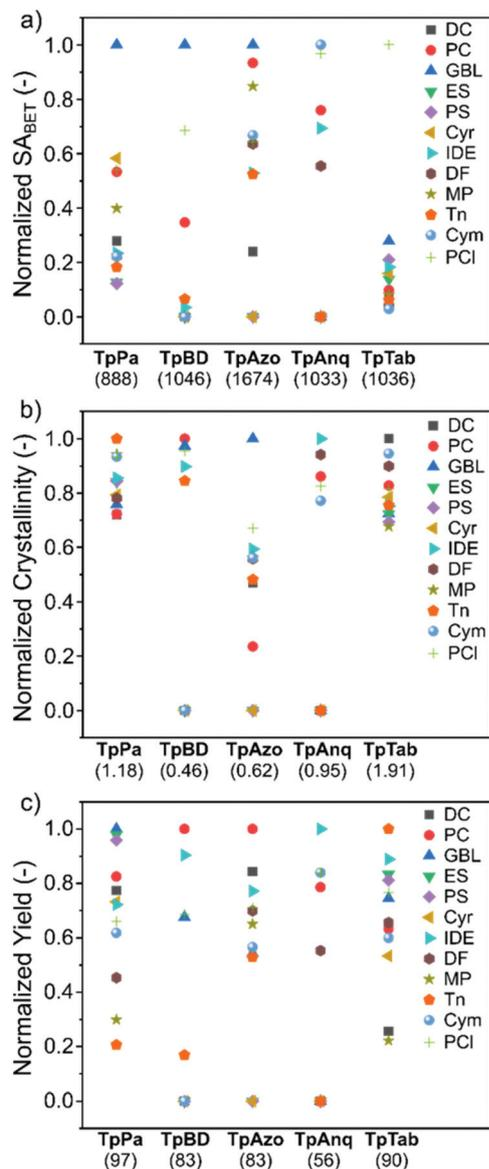
Fig. 4 (a) Relative surface area, (b) relative crystallinity, and (c) relative yield of the TpPa, TpBD, TpAzo, TpAnq, and TpTab series of COFs synthesized in twelve green solvents. The value provided in parenthesis along the x-axis denotes the maximum value of (a) BET surface area ( $\text{m}^2 \text{g}^{-1}$ ), (b) crystallinity, and (c) yield (%) used in the calculations (section S4, ESI†).
