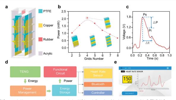
Fig. 5 TENGs as sustainable power sources for heart rate monitoring. (a) Schematic illustration of the device structure of the D-TENG. (b) Output power of the D-TENG with different grid numbers under a consistent mechanical excitation of 10 Hz. (c) Heart-rate signal acquired by the BSN with an integrated D-TENG. (d) System diagram of the complete power-supplying system. (e) Enlarged view to show the whole software interface of the real-time acquired heart-rate signals.<sup>59</sup>
