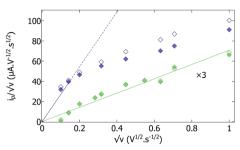
Fig. 2 Evaluation of the thin (green, enlarged three times) and thick (dark blue) hydrogenase/polymer films by cyclic voltammetry under non-catalytic conditions (under argon). Plot of anodic (open) and cathodic (full) peak currents divided by the square root of scan rate ( $\sqrt{\nu}$ ), against  $\sqrt{\nu}$ . A straight line through the origin is expected when the film is so thin that all viologen moieties are oxidized or reduced in each sweep.
