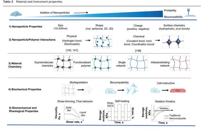
The table displays the important properties of bioinks, biomaterial inks, as well as bioprinters. Nanomaterial reinforcement helps improving the printability of traditional hydrogels. However, the material must be biocompatible. Additionally, the table shows significant considerations for the nanoparticle type, nanoparticle/polymer interaction, material chemistry, printing parameters, rheological and biomechanical properties, and biochemical properties.
