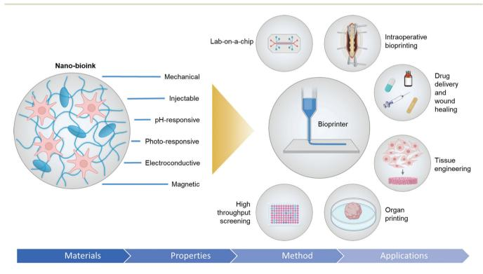
Fig. 1 Multifunctionalities of nanocomposite hydrogel-based bioinks. Schematic highlights the different functionalities of a bioink imparted by nanoparticles. It also demonstrates the possible applications of nanocomposite hydrogel-based bioinks.
