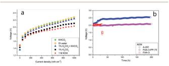
Fig. 7 (a) Polarization curves recorded for different electrolytes and (b) stability of various MEAs: A201, FAA-3, and FAA-3-PP-75. Reprinted from ref. 55 with permission from Elsevier.
