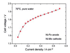
Fig. 3 Cell performance of the first prototype of an AEM water electrolysis system using Ni-Fe anode and Ni-Mo cathode and working only with pure water.33 Reproduced from ref. 33 with permission. Copyright@2014. Royal Society of Chemistry.
