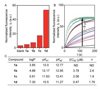
Fig. 2 Comparison of ion transport activity of compounds 1a-1d (0.5 μM) at 200 seconds across EYPC-LUVs⊃HPTS (A). Concentration profile of compound 1d (B); and correlation table for the estimated logP and p $K_a$  values with experimentally determined EC<sub>50</sub> and Hill coefficient (n) values (C).
