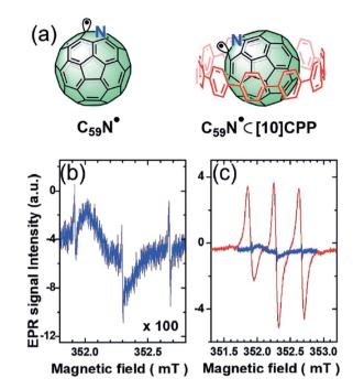
Fig. 8 (a) The structures of  $C_{59}N^*$  and  $C59N^* \subset [10]$ CPP. (b) The ESR signal of  $C_{59}N^*$ . (c) The comparison of the ESR signal of  $C_{59}N^*$  and  $C59N^* \subset [10]$ CPP. Reproduced from ref. 54 with permission from Wiley-VCH, Copyright 2019.
