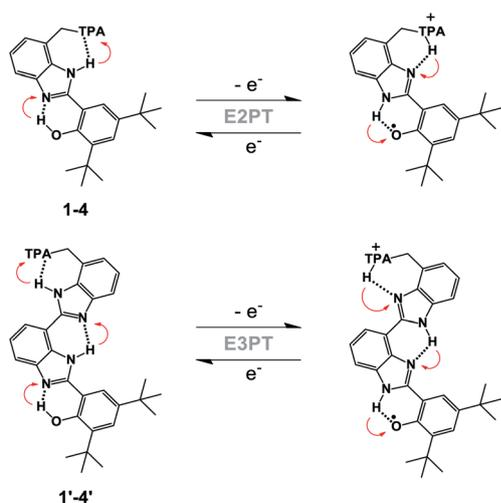
Fig. 2 Generic structure of BIP derivatives **1**–**4** (top), and BI<sub>2</sub>P analogs **1'**–**4'** (bottom) showing the electrochemical oxidation of the phenol coupled with two (E2PT) or three (E3PT) proton transfers. Red arrows indicate proton movement for the forward and reverse processes.
