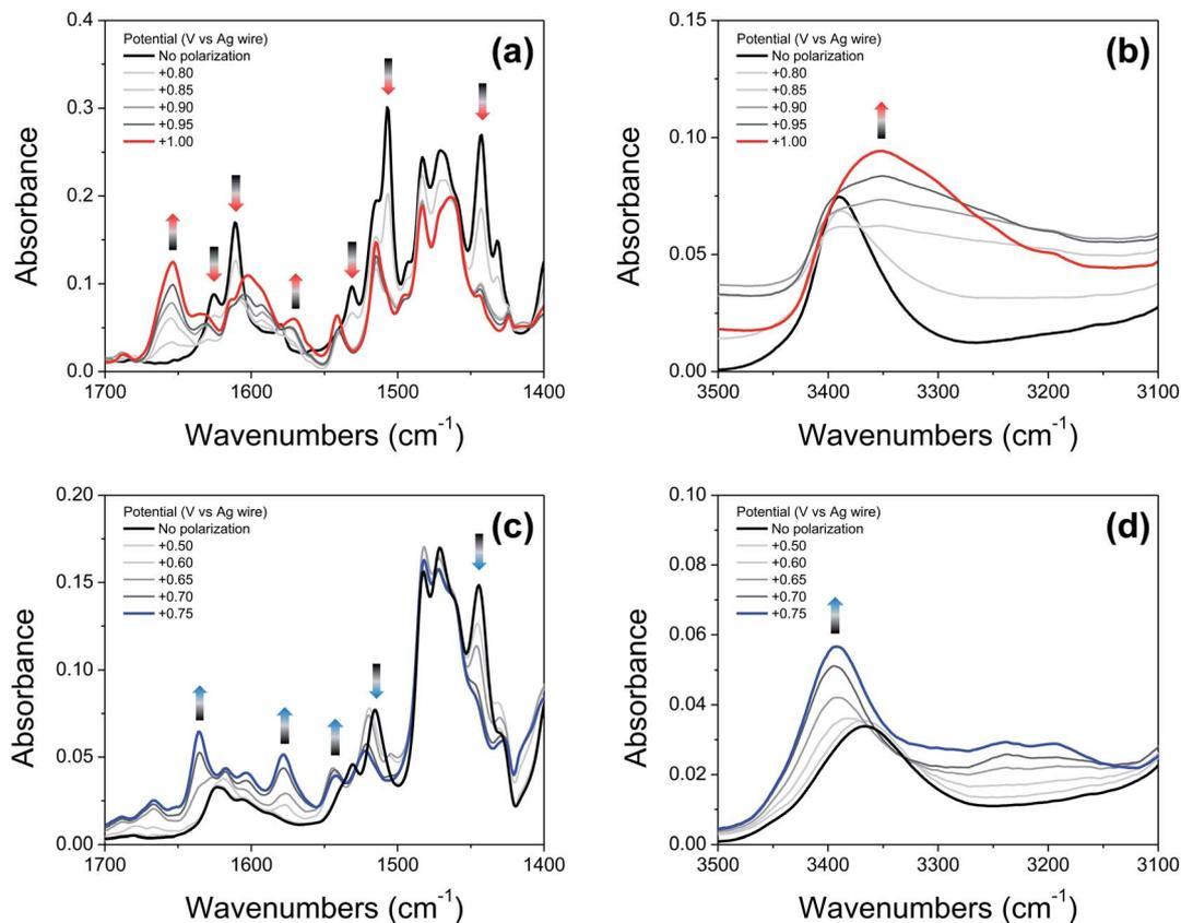
Fig. 6 (a and c): IRSEC spectra of **2'** and **4'**, respectively, (19 mM solutions) polarized in 50 mV or 100 mV steps in the 1700–1400  $\text{cm}^{-1}$  region. (b and d): IRSEC spectra of **2'** and **4'**, respectively, under the same conditions in the 3500–3100  $\text{cm}^{-1}$  region. Solvent: DCM, 0.1 M TBAPF<sub>6</sub>. Some of the characteristic bands showing changes upon electro-oxidation are indicated with upward and downward arrows.
