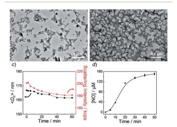
Fig. 3 TEM images of aqueous dispersions (0.1 g  $L^{-1}$ ) of BP1 vesicles (a) before and (b) after UV 365 nm irradiation. (c) Evolution of hydrodynamic diameters,  $\langle D_h \rangle$ , and corresponding scattering intensities and (d) NO release profile of BP1 vesicles under UV 365 nm irradiation (4 mW cm<sup>-2</sup>). Data represent mean  $\pm$  s.d. (n = 3).
