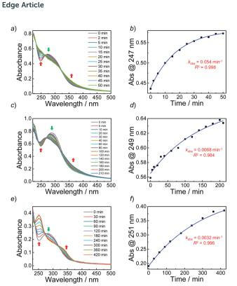
Fig. 4 (a, c and e) Absorbance spectra and (b, d and f) absorbance intensity changes together with a mono-exponential fit of aqueous dispersions (0.1 g L $^{-1}$ , 25 °C) of (a and b) BP1 vesicles, (c and d) BP2 vesicles, and (e and f) BP3 micelles under UV 365 nm irradiation (4 mW cm $^{-2}$ ).
