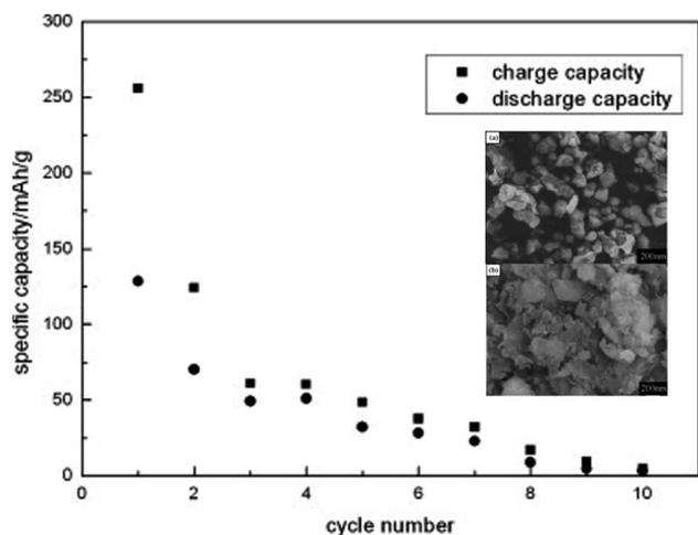
Fig. 16 Cyclic performance of  $\text{Li}_2\text{MnSiO}_4$  synthesized by solid state method tested at C/16 rate to a cut-off voltage between 1.5 and 4.8 V.<sup>152</sup> The inset shows FESEM micrographs of (a)  $\text{Li}_2\text{MnSiO}_4$  and (b)  $\text{Li}_2\text{MnSiO}_4/\text{C}$ .
