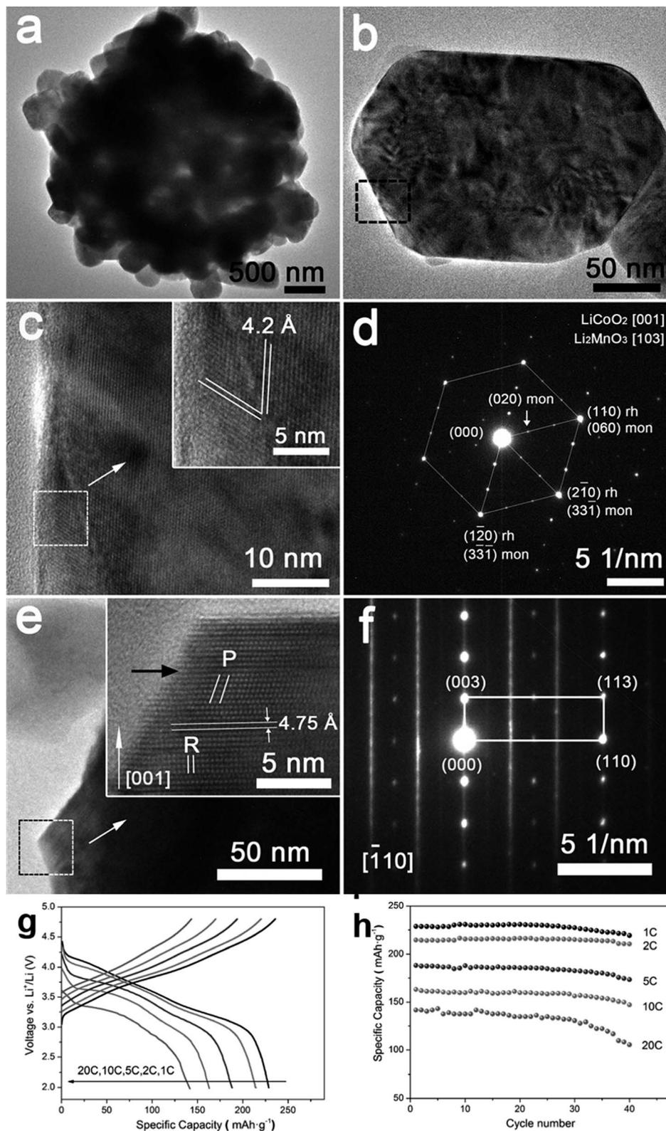
**Fig. 8** (a–f) Hierarchical  $\text{Li}_{1.2}\text{Ni}_{0.2}\text{Mn}_{0.6}\text{O}_2$  nanoplates with exposed  $\{010\}$  planes as high-performance cathode material for lithium-ion batteries, (g) discharge curves of half cells based on the  $\text{Li}_{1.2}\text{Ni}_{0.2}\text{Mn}_{0.6}\text{O}_2$  hierarchical structure nanoplates at 1C, 2C, 5C, 10C, and 20C rates after charging at C/10 rate to 4.8 V, and (h) the rate capability at 1C, 2C, 5C, 10C, and 20C rates.<sup>88</sup>
