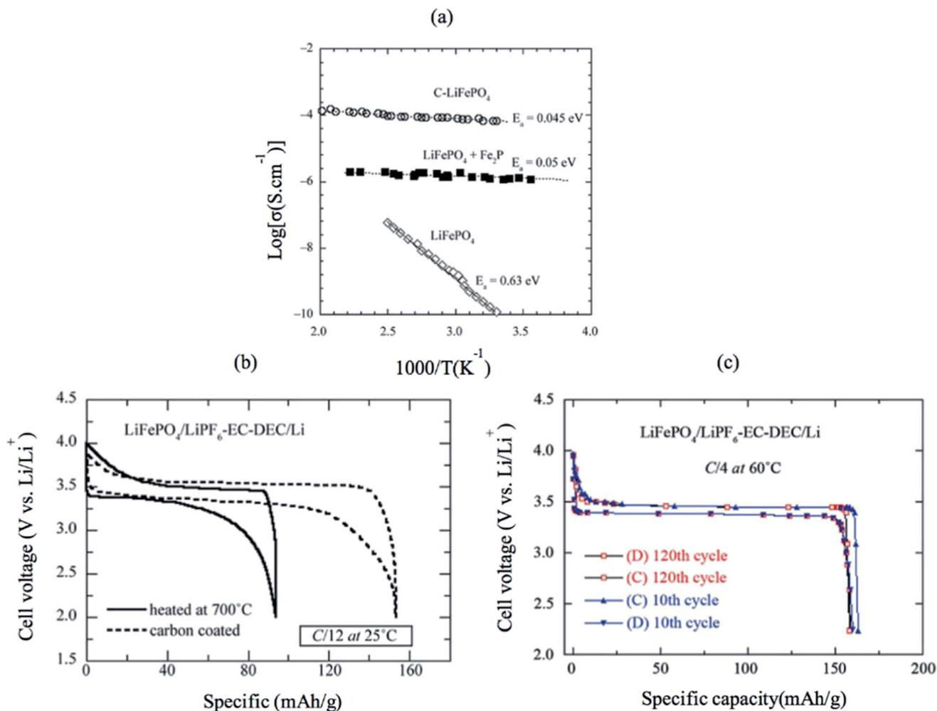
Fig. 12 (a) Electronic conductivity of pure LiFePO<sub>4</sub>, Fe<sub>2</sub>P-containing sample and C/LiFePO<sub>4</sub>. (b) The electrochemical profiles at C/12 of non-coated and heated at 700 °C LiFePO<sub>4</sub>//Li cells (c) electrochemical performance of the C-LiFePO<sub>4</sub>//Li cell operating at 60 °C. Charge–discharge cycling was conducted at the C/4 rate (about 35 mA g<sup>-1</sup>) in the voltage range 2.2–4.0 V vs. Li<sup>0</sup>/Li<sup>+</sup>.<sup>123</sup>
