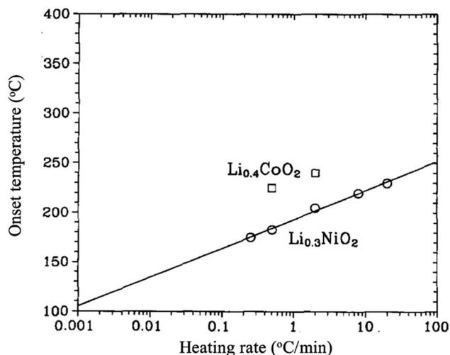
Fig. 6 The onset temperature for oxygen release for  $\text{Li}_{0.3}\text{NiO}_2$  and  $\text{Li}_{0.4}\text{CoO}_2$  as a function of heating rate.<sup>35</sup>
