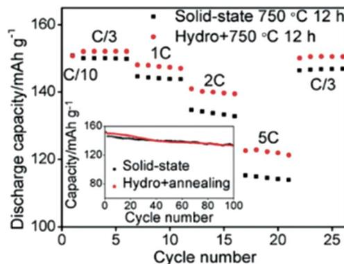
Fig. 19 Comparison of two materials, one was sintered for 12 h at 750 °C and the other was prepared by hydrothermal method then sintered for 12 h at 750 °C.<sup>159</sup>
