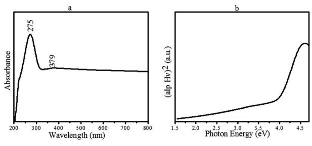
Fig. 7 (a) UV-Vis absorption spectra of CoMoO<sub>4</sub>, and (b) band gap energy of CoMoO<sub>4</sub> via Tauc's plot.
