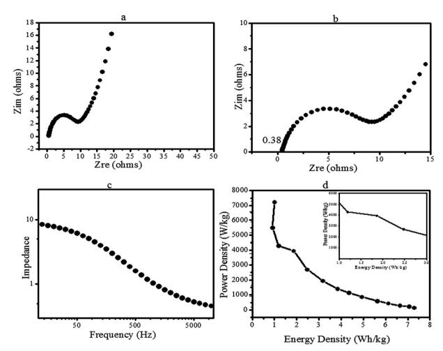
Fig. 9 (a) Nyquist plot of  $CoMoO_4$  in the low frequency region, (b) Nyquist plot (semicircle arc) in the high-frequency region, (c) variation of impedance as a function of frequency, and (d) Ragone plot of  $CoMoO_4$  (inset depicts the response of the energy density at higher power density).
