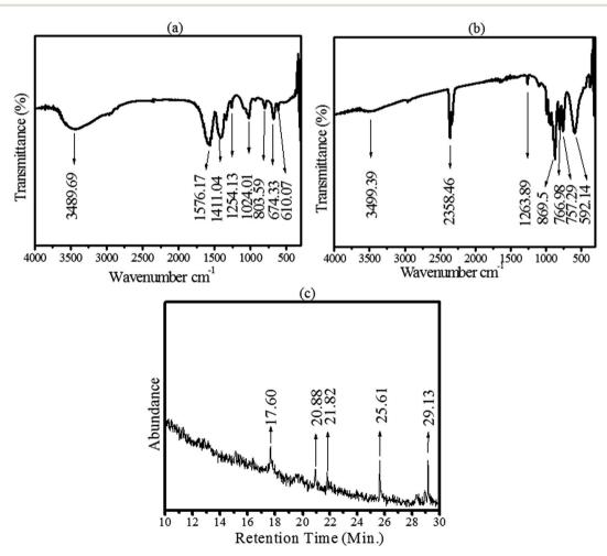
Fig. 2 Identification of organic stabilizing agents of CoMoO<sub>4</sub>. (a) FTIR spectra of CoMoO<sub>4</sub> after drying at 95 °C. (b) FTIR of CoMoO<sub>4</sub> after annealing at 450 °C, and (c) GC-MS spectra of CoMoO<sub>4</sub>.
