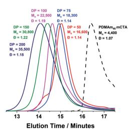
**Fig. 5** DMF GPC chromatograms for a series of PDMAm<sub>46</sub>-b-PDAAm<sub>y</sub> polymer nano-objects synthesised in a tubular reactor where y=50 to 200. Reactions were conducted at 90 °C using RAFT aqueous dispersion polymerisation at 20% w/w solids and [PDMAm<sub>113</sub>]: [VA-044] = 50:1. GPC data was calibrated against a series of ten near-monodisperse poly (methyl methacrylate) standards.
