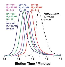
Fig. 3 DMF GPC chromatograms for a series of PDMAm<sub>113</sub>-b-PDAAm<sub>v</sub> block copolymers synthesised in a flow reactor where y = 50 to 200. Polymerisation was conducted at 90 °C, 20% w/w solids and [PDMAm<sub>113</sub>]: [VA-044] = 50:1. GPC data was calibrated against a series of ten near-monodisperse poly(methyl methacrylate) standards.
