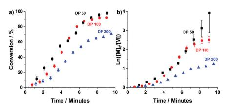
Fig. 2 (a) Conversion vs. time and (b) semi-logarithmic rate plots for the continuous-flow RAFT aqueous dispersion polymerisation of diacetoneacrylamide (DAAm) using a PDMA $m_{113}$  macro-CTA targeting PDAAm DPs of 50, 100 and 200. All reactions were conducted at 90 °C with total solids concentration of 20% w/w and [PDMA $m_{113}$ ]: [VA-044] = 1:0.02.
