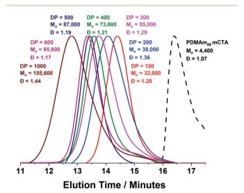
Fig. 7 DMF GPC chromatograms for a series of PDMAm<sub>46</sub>-b-PDAAm<sub>y</sub> polymer nano-objects synthesised in a tubular flow reactor where y =150 to 1000. Polymerisation was conducted at 70 °C using RAFT aqueous dispersion polymerisation at 20% w/w solids and [VA-044] = 0.25 mM. GPC data was calibrated against a series of ten near-monodisperse poly(methyl methacrylate) standards.
