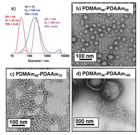
Fig. 6 (a) DLS traces for PDMAm $_4$ 6-b-PDAAm $_y$  polymer nano-objects and representative transmission electron microscopy images for pure sphere morphologies block copolymers where y = (b) 50, (c) 75, (d) 100. All images were obtained from 0.1% w/w aqueous dispersions of diblock copolymer at pH 3.
