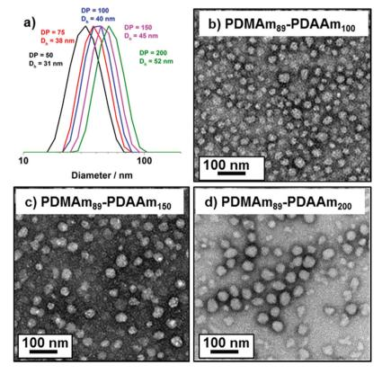
Fig. 4 (a) DLS traces for PDMAm<sub>113</sub>-b-PDAAm<sub>v</sub> polymer nano-objects and representative TEM images for pure sphere morphologies block copolymers where y = (b) 100, (c) 150, (d) 200. All images were obtained from 0.1% w/w aqueous dispersions of diblock copolymer at pH 3.
