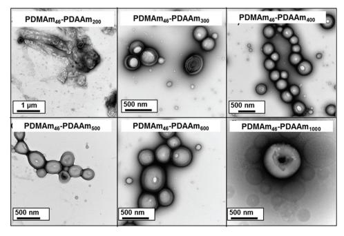
Fig. 8 Representative transmission electron microscopy images of PDMAm<sub>46</sub>-b-PDAAm<sub>v</sub> block copolymers, synthesised in the flow reactor, where y = (a) 200, (b) 300, (c) 400, (d) 500, (e) 600 and (f) 1000. All images were obtained using 0.1% w/w of diblock copolymer at pH 3.
