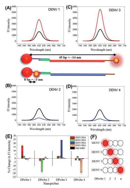
Fig. 5 Distance-dependent fluorescence intensity changes of CdSeTeS QDs of the four different sensing nanoprobes in the presence of four different analytes of DENV 1 (A), DENV 2 (B), DENV 3 (C) and DENV 4 (D) serotypes. (E) Comparative bar diagram for the cross sensitivity of all four nanoprobes in the presence of all four types of DENV serotypes. (F) Pictorial illustration of the cross-reactivity determination of the sensor.
