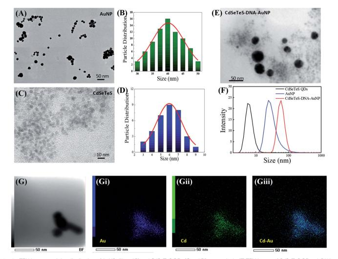
Fig. 2 TEM images and size distribution of AuNPs (A and B) and CdSeTeS QDs (C and D), respectively. (E) TEM image of CdSeTeS QDs – dsDNA – AuNPs, (F) DLS hydrodynamic sizes of CdSeTeS QDs, AuNP and CdSeTeS QDs-dsDNA-AuNP nanocomposites, and (G) STEM mapping of CdSeTeS QDs-dsDNA-AuNP, (Gi) Au, (Gii) Cd and (Giii) merged image.
