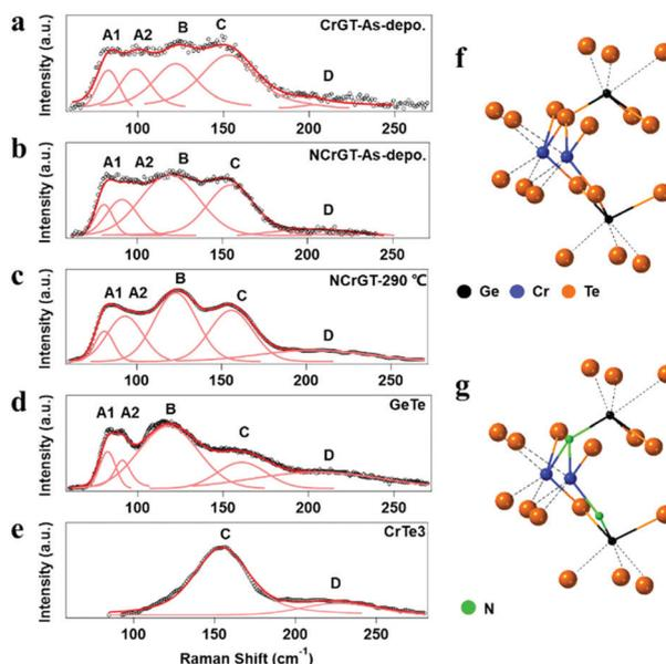
Fig. 2 Raman spectra of amorphous (a) as-deposited CrGT, (b) as-deposited NCrGT, (c) 290 °C-annealed NCrGT, (d) as-deposited GeTe, and (e) as-deposited CrTe<sub>3</sub> films with corresponding Gaussian fitting. The schematic local structures of the as-deposited amorphous (f) CrGT and (g) NCrGT.
