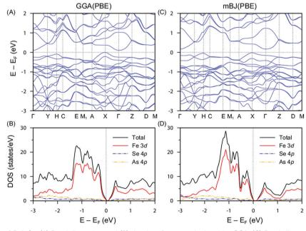
Fig. 7 Electronic structure of FeAsSe. (A) Band dispersion and (B) density of states calculated by GGA. (C) Band dispersion and (D) density of states calculated by mBJ.
