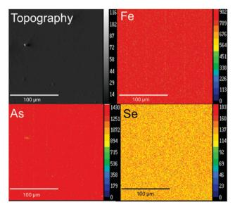
Fig. 3 Topological and X-ray elemental maps of single crystal FeAs<sub>1,50</sub>Se<sub>0,50</sub>
