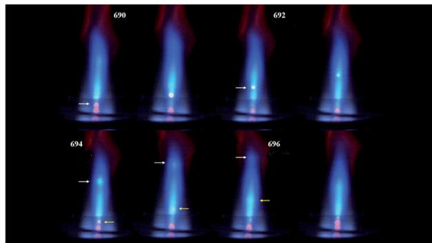
Fig. 1 Successive frames from a small section of Video 1.† Frame 690 is the first image from this clip. Alternate frames are numbered in the order they were measured. The time interval between frames was 200  $\mu\text{s}$ . A white arrow pointing right denotes the first droplet cloud under discussion. The yellow arrow pointing left denotes the second such droplet.
