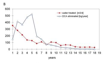
Fig. 2 Full scale treatment of 1,2-dichloroethane-contaminated groundwater. (A) Rotating biological contactor with biofilm containing the yellow-pigmented DCA degrader *Xanthobacter autotrophicus* GJ10. (B) Performance of the system over an 18 year period.
