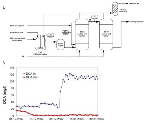
Fig. 3 Full scale treatment of 1,2-dichloroethane-contaminated groundwater in a packed bed bioreactor. (A) Process scheme. (B) Influent and effluent concentrations after startup.
