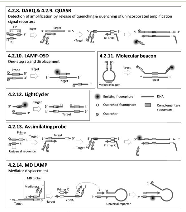
Fig. 5 Schematic illustrations of 4.2.8. DARQ LAMP<sup>68</sup> & 4.2.9. QUASR LAMP,<sup>73</sup> 4.2.10. LAMP-OSD,<sup>83</sup> 4.2.11. molecular beacon,<sup>88</sup> 4.2.12. Light-Cycler, 94 4.2.13. assimilating probe96 and 4.2.14. MD LAMP101 (redrawn according to the references).
