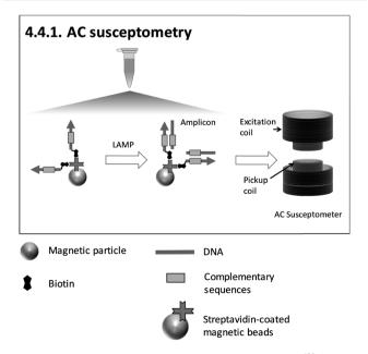
Fig. 8 Schematic illustration of 4.4.1. AC susceptometry  $^{150}$  (redrawn according to the references).
