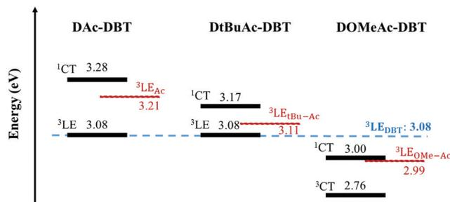
Fig. 6 A schematic energy diagram of **DAC-DBT**, **DtBuAc-DBT** and **DOMeAc-DBT**. All energies are given in eV and were calculated from the onsets of the corresponding spectra in zeonex films, compared with their individual D and A moieties. No indication of  $^3\text{CT}$  states is obtained in **DAC-DBT** and **DtBuAc-DBT** from calculations, neither are they observed in our experiments, therefore, their  $^3\text{CT}$  states are not represented in this diagram.
