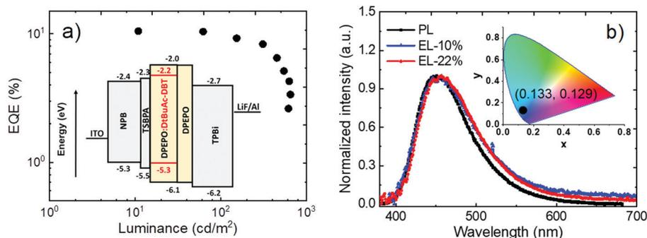
Fig. 9 (a) EQE vs. luminance characteristics. Inset shows the device structure and energy levels. (b) The comparison of PL spectrum of DPEPO:10%**DtBuAc-DBT** film and EL spectra of 10% and 22% doping concentration in blue devices collected at 9 V. The inset shows the CIE coordinates of the devices.
