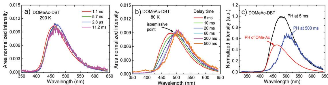
Fig. 8 **DOMEAc-DBT** in zeonex film: time-resolved area normalized emission spectra at (a) 290 K and (b) 80 K. (c) Phosphorescence spectra recorded at delay times of 5 ms and 500 ms, compared with the that of the donor OMe-Ac unit measured at 80 K.
