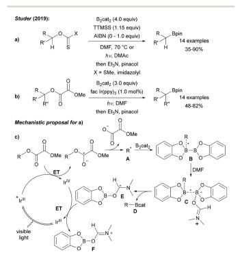
Scheme 18 Radical borylation of secondary (a) and tertiary (b) alcohols via its xanthates, thionocarbamates and methyl oxalate esters. Mechanism (c).
