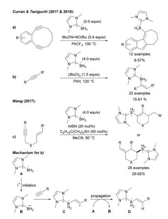
Scheme 29 Radical C-B bond formation by intermolecular addition of NHC boryl radicals to alkynes and alkenes. Transannular cyclisation (a), alkyne (b) and enyne (c) hydroboration. Mechanism (d).
