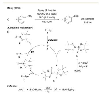
Scheme 1 Metal free borylation of anilines *via in situ* generation of diazonium salts (a). Mechanism (b).
