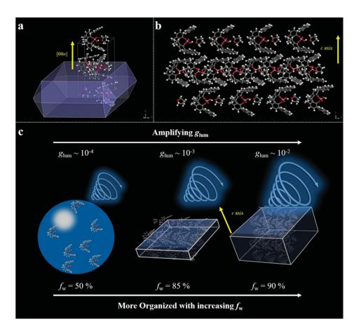
Fig. 5 Molecular packing analysis results and speculated mechanism for the amplification of  $g_{lum}$ . (a) Theoretically predicted growth morphology of an S-SPAn crystal based on the attachment energies calculated with Material Studio package. (b) Crystal packaging along the vertical growth direction. (c) Speculated mechanism for the amplification of  $g_{lum}$ .
