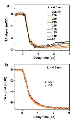
Fig. 3 (a) Hot exciton relaxation dynamics (monitored at B1) for  $L=4.3\,$  nm NCs at varying temperatures. (b) Hot exciton relaxation dynamics (monitored at B1) for  $L=4.3\,$  nm pristine NCs (with OA ligands; orange diamonds) and DDT-capped NCs (wine circles).
