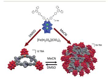
Fig. 8 Schematic illustration of the formation of two types of nanostructures by complexation of  $TBA_6[P_2W_{17}O_{61}(O(Si-C_{29}H_{18}N_3)_2)]_3$  with Fe<sup>2+</sup> ions. Colour code: W, blue polyhedra or spheres; P, green polyhedra; Si, yellow; N, violet; C, gray; O, red spheres. Adapted with permission from ref. 54. Copyright 2016 American Chemical Society.
