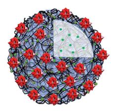
Fig. 10 The POM coacervate vesicle formed by the Keggin-type  $[PW_{11}O_{39}]^{7-}$  units, ATP (green spheres) and PDDA (black bent lines). Colour code: W, red polyhedra; P, blue spheres. Adapted with permission from ref. 65. Copyright 2014 of Wiley-VCH Verlag GmbH &
