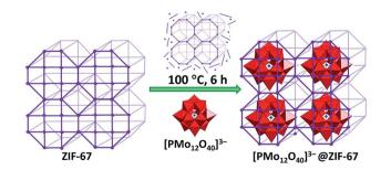
Fig. 4 Schematic depiction of the synthetic procedure used for the preparation of the hybrid  $[PMo_{12}O_{40}]^{3-}$ @ZIF-67. Colour code: W, red polyhedra; P, blue spheres. Adapted from ref. 41, with permission from The Royal Society of Chemistry.
