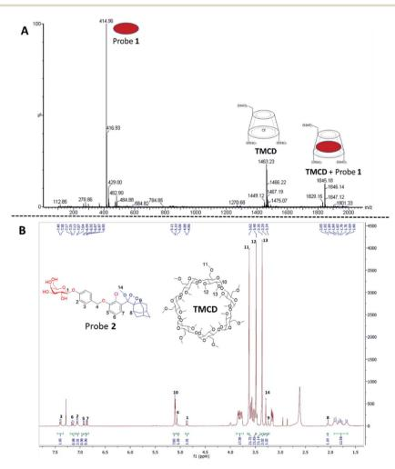
Fig. 4 (A) Negative ESI spectra of an aqueous solution of probe 1 and TMCD prepared in a 1:1 molar ratio. (B)  $^1$ H-NMR spectrum of the crystalline supramolecular complex of probe 2 with TMCD. The crystallization experiment was carried out in H<sub>2</sub>O: DMF (95:5) with probe 2 and TMCD mixed at an initial molar ratio of 1:5.
