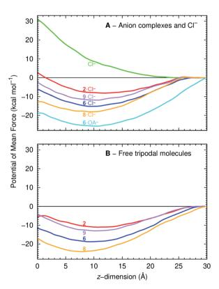
Fig. 10 PMF as a function of anionophore distance to the membrane centre of mass (z=0 Å), for the Cl $^-$  complexes (top) and free transporters (bottom). The red, blue, purple and orange lines correspond to 2, 6, 9 and 8. The green line corresponds to the PMF of a free Cl $^-$  and the cyan line to the PMF of 6  $\cdot$  OA $^-$ .
