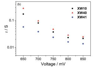
Fig. 7 Plots of (a)  $C_{\mu}$  and (b)  $\tau$  versus bias voltages of DSSCs based on XW10, XW40, and XW41.
