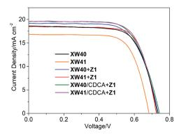
Fig. 5 J-V characteristics of the DSSCs based on Z1, XW40 and XW41.
