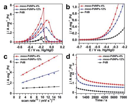
Fig. 6 (a) Mass-normalized cyclic voltammograms (CVs), (b) linear sweep voltammograms (LSVs), and (d) chronoamperometric curves (recorded at -0.2 V) for EOR in 1.0 M NaOH containing 1.0 M C<sub>2</sub>H<sub>5</sub>OH. (c) The relationship of peak current density *versus* the square root of the scan rate. The CV and LSV curves were obtained at a scan rate of 50 mV s<sup>-1</sup> and 1 mV s<sup>-1</sup>, respectively.
