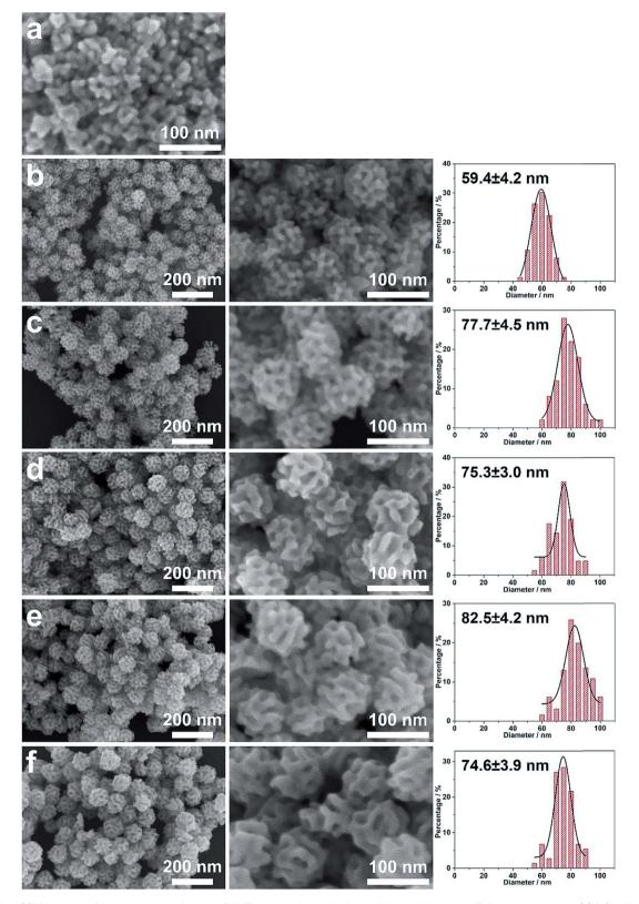
Fig. 4 Typical SEM images of the as-prepared meso-PdNPs under the typical conditions with various Pd concentrations: (a) 1.6 mM, (b) 3.2 mM, (c) 4.8 mM, (d) 9.6 mM, (e) 12.8 mM, and (f) 16.0 mM, respectively. The histograms on the right side show the distribution of the corresponding particle sizes.
