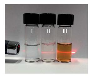
Fig. 2 Photo showing the Tyndall effect in solutions with different compositions: (i) PS-b-PEO dissolved in THF, (ii) PS-b-PEO dissolved in H $_2$ O mixed with 4% THF, and (iii) PS-b-PEO dissolved in H $_2$ O mixed with 4% THF + H $_2$ PdCl $_4$ .
