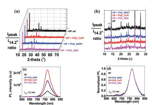
Fig. 2 Crystallographic and optical characterization of perovskite films without (HP) and with PbS QDs (50  $\mu$ g ml<sup>-1</sup>) deposited on glass of PbS QDs with the different capping ligands including MAPI, CsPI and 4-aminobenzoic acid (ABA). XRD spectra (a) and a zoom-in from 10 to 35° (b) (the \* symbol indicates the PbI<sub>2</sub> diffraction peak); (c) photoluminescence (PL) and (d) normalized PL spectra.
