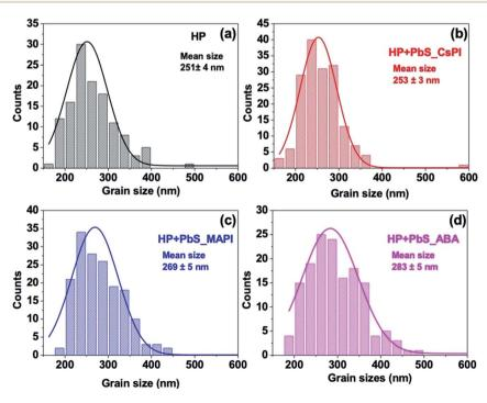
Fig. 1 Grain sizes of perovskite estimated from SEM images of (a) perovskite films without (HP) and with PbS QDs (50  $\mu$ g ml<sup>-1</sup>) deposited on glass of PbS QDs with the different capping ligands including (b) MAPI, (c) CsPbI and (d) 4-aminobenzoic acid (ABA).
