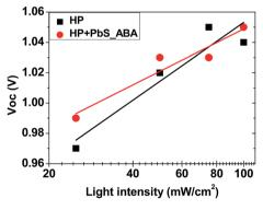
Fig. 5 Dependence of open circuit voltage on light intensity for the champion cells (see Table 2) with the architecture FTO/SnO<sub>2</sub>/ absorber/spiro-OMeTAD/Au, in which absorber layers were perovskite films without (HP) and with PbS QDs (50  $\mu$ g ml<sup>-1</sup>) and PbS QDs had the 4-aminobenzoic acid (ABA) ligand. The measurement was done at room temperature.
