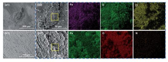
Fig. 9 The SEM morphological images of corrosion products on the substrate coated with (a1 and a2) pure EP and (b1 and b2) 0.5% N-CDs-EP after 70 days of immersion. EDS is shown in the blue box.
