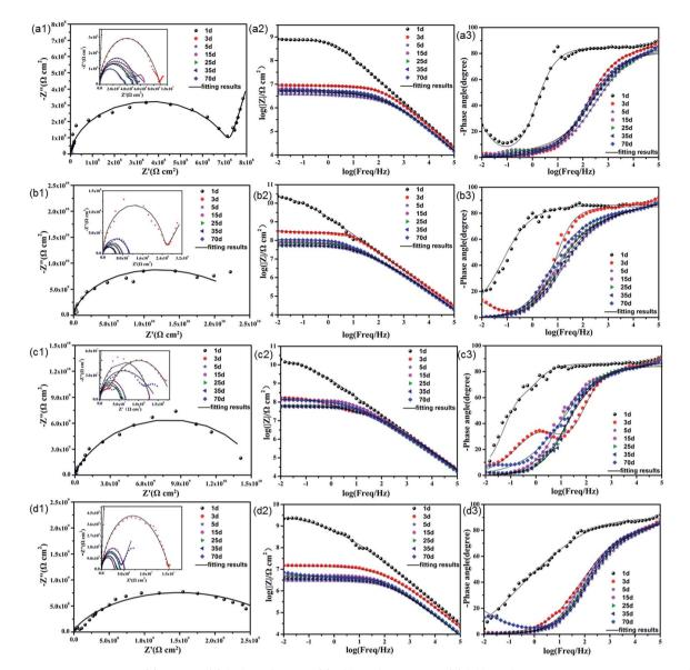
Fig. 7 Nyquist and Bode plots of (a) pure EP; (b) 0.5% N-CDs-EP; (c) 1.0% N-CDs-EP; and (d) 2.0% N-CDs-EP coatings immersed in 3.5% NaCl solution during 70 days (solid lines indicate fitting data)
