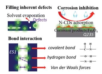
Fig. 11 Corrosion resistance mechanism of the N-CDs-EP coating.
