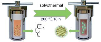
preparation of N-CD 1 Schematic illustration of the nanomaterials.
