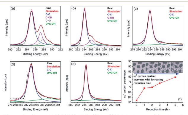
Fig. 1 XPS spectra of the rGO sample for (a) 0 h (GO), (b) 1 h, (c) 2 h, (d) 3 h, and (e) 5 h of reduction treatment. (f) Shows the variation of sp<sup>2</sup> carbon as a function of reduction time. The inset to (f) is a structural model of GO at various steps of the reduction process. Here, dark areas indicate sp<sup>2</sup> carbon domains, and light grey areas are sp<sup>3</sup> carbons consisting of oxygen groups (depicted as small dots). Reproduced with permission from ref. 18.
