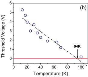
Fig. 4 (a) Temperature dependent I-V plots of the sensor in the bias range from -20 V to +20 V. (b) Threshold voltage ( $V_{\text{Th}}$ ) as a function of temperature.
