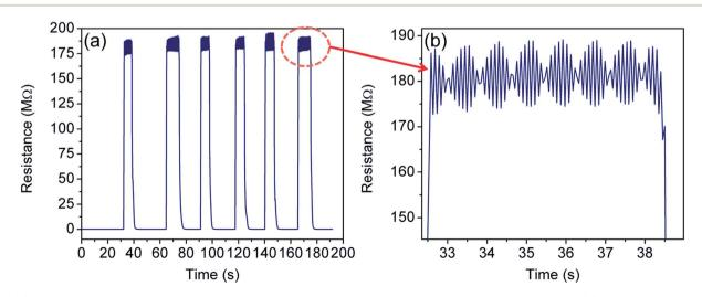
Fig. 9 (a) Sensor response when the sensor is frequently dipped into liquid nitrogen for short time durations, and (b) zoomed in image of the highlighted spot in (a) showing the formation of the oscillatory pattern (in the form of an envelope) at 77 K.
