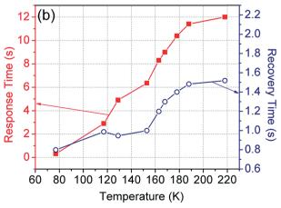
Fig. 7 (a) Sensor operation at a specific temperature by exposing (or removing) it to a target temperature from room temperature, and (b) the corresponding response and recovery time of the sensor.
