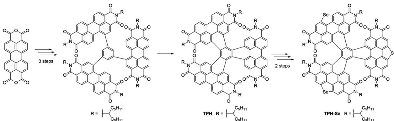
**Fig. 11** Synthetic routes employed for **TPH** and **TPH-Se** involving photocyclization to achieve a fully-annulated aromatic core.
