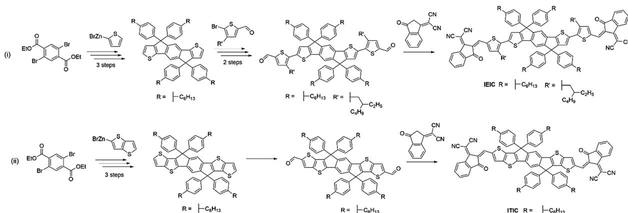
Fig. 7 Comparison of the synthetic routes required for (i) IDT based **IEIC** and (ii) IDTT based **ITIC**.
