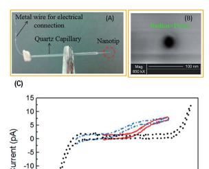
Fig. 5 (A) Photograph and (B) scanning electron micrograph of a nanopipette prepared by a laser-pulled capillary. (C) Cyclic voltammogram of 2 mM acetylcholine (ACh), tetraethylammonium (TEA), and artificial seawater (ASW). TEA was used as an internal standard and ASW was the solvent (background signal). Adapted with permission from Colombo et al.81
