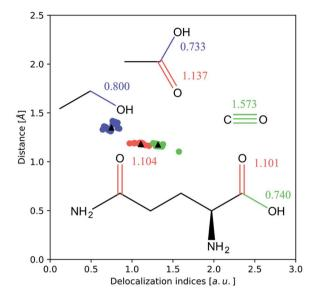
Fig. 3 k-Means clustering of the internuclear distance d versus  $\delta$  plot for carbon-carbon (left) and carbon-oxygen (right) bonds (interactions smaller than 0.5 a.u. have been removed). The vast majority of examples are concentrated in a band between 1.0 and 2.0 Å, and correspond to the single, double and triple bonds for carbon-carbon interactions, and to the single and double bonds for carbon-oxygen interactions.
