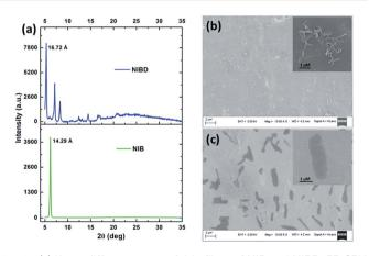
Fig. 4 (a) X-ray diffractograms of thin films of NIB and NIBD. FE-SEM images of NIBD (b) and NIB (c) formed by the evaporation of the respective aggregates from a 99.9% water–0.1% DMF mixture on aluminium foil at room temperature (10  $\mu$ M).
