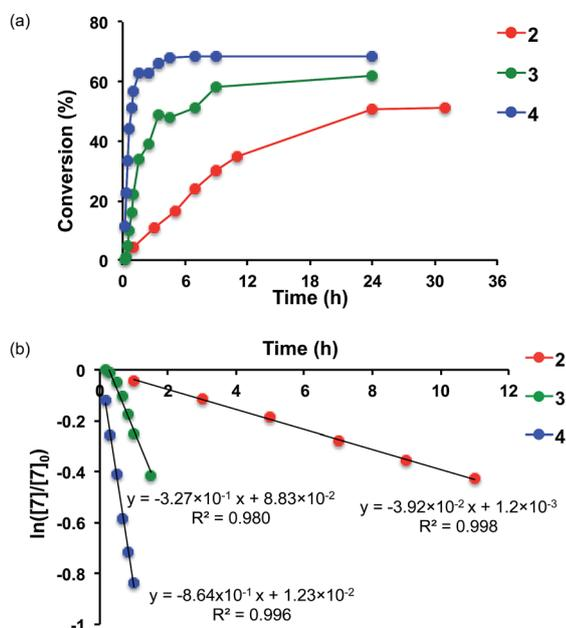
Fig. 5 (a) Plot of conversion vs. time for RCM of **7** to **8** using catalysts **2–4**. (b) Plot of  $\ln([7]/[7]_0)$  vs. time for this reaction. Conversion determined by  $^1\text{H}$  NMR. Selectivity determined using gas chromatography.
