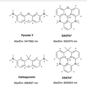
Chart 2 Chromophore analysis of Pyronin Y, carbopyronin, DAOTA<sup>+</sup>, and CDATA<sup>+</sup>. The values of the lowest energy absorption maximum (Abs) and emission maximum (Em) are from this work and ref. 7.
