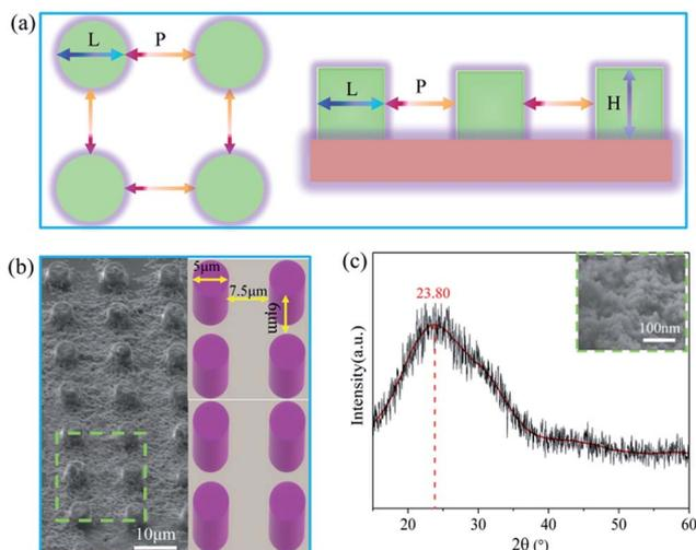
Fig. 2 (a) The top view (left) and side view (right) of the MPA. This pattern was repeated periodically across the PDMS surface. (b) The FESEM image of the fabricated SiO<sub>2</sub>-sprayed MPA under low-magnification, demonstrating that the coated PDMS has a negligible effect on the global structure of the MPA. (c) The X-ray diffraction (XRD) spectrum of the coating and high-magnification FESEM image shows the nanoscale SiO<sub>2</sub> (insert).
